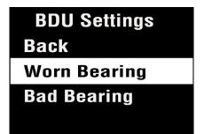
The BDU threshold values are designated as Worn Bearing (where readings turn Amber) and Bad Bearing (where readings turn Red).
