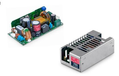
The new TOP-100 Series AC/DC Power Supplies feature the highest power rating in the industry standard  $2.0'' \times 4.0''$  (50.8 x 101.6 mm) footprint. They can supply up to 100 W output power with convection cooling over an industrial operating temperature range of  $-25^{\circ}$ C to  $+50^{\circ}$ C. This performance could be realized by a state of the art design providing an extremely high efficiency of >90 % which eliminates the need for a dedicated power supply cooling fan.
